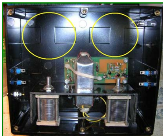
Single bank of plate capacitor tuners, silver Sephorah radio coil and solid state amplification visible pre-wiring. Yellow circles show approx. location of input and output wells.
